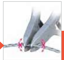
Do Not Bend Repeatedly (Can Weaken Plate)
